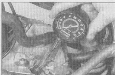
3.20 Using a rubber-cone type cylinder compression gauge
