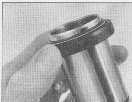
8.22 Install the oil seal
