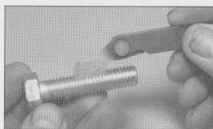
2.12 Using a thread gauge to measure pitch
