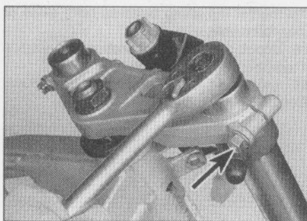
7.11 If the forks are going to be disassembled, loosen the upper clamp bolt, then loosen the top plug with a 1/2 inch drive ratchet
